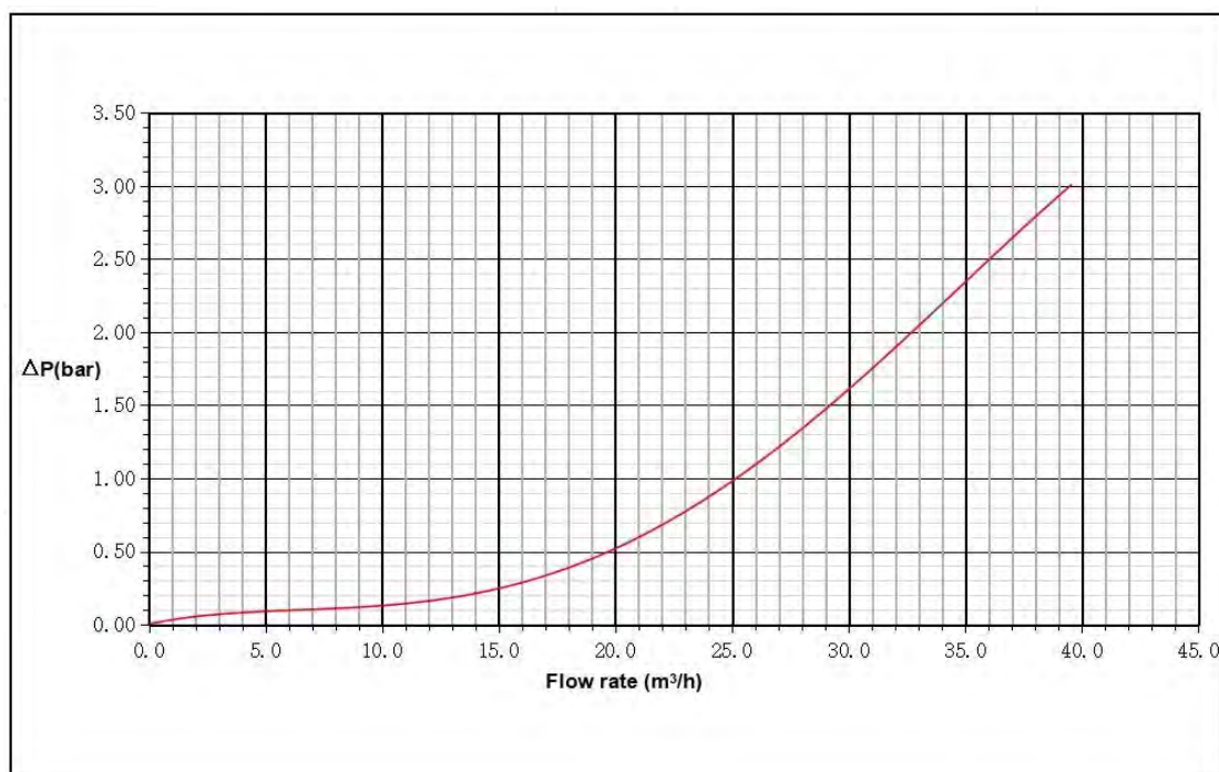
Figure 2 - Pressure loss curve - Backwash mode
