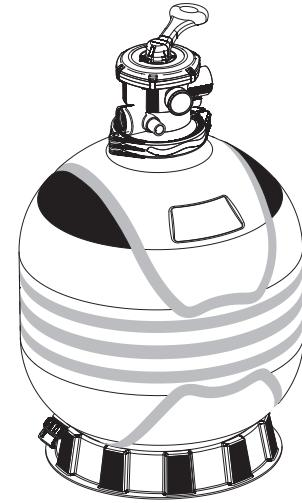
operation will depends on how dirty your filter is. Check the sight glass to see when the water becomes clear. It is recommended that the backwash should be at least 2 minutes long.
